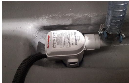
12 V electric bilge pump
